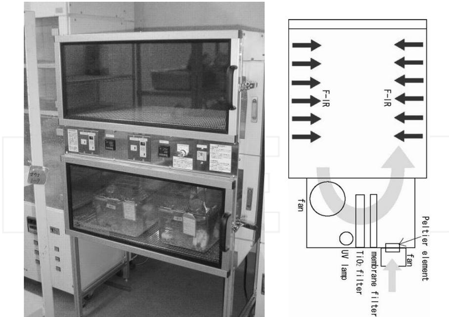
**Figure 8.** The FIR animal raising apparatus
